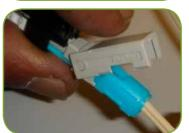
• Push the lever down to lock the cable clamp to the main body of the connector until a "click" is heard indicating a successful operation
