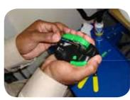
• Install SC/APC connector to individual fibre
