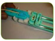
• Mount the cable holder assembly into the mechanical stripper cradle as shown
