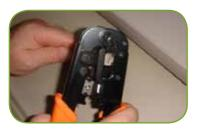
• With the wires fully inserted into the connector, place the assembly into the crimp tool. Make sure the connector is fully inserted into the crimp tool before crimping
