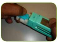
• Press and hold the jaws of the mechanical stripper firmly before pulling the cradle assembly to the side to carry out the stripping operation
