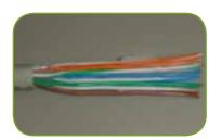
• Arrange the pairs into correct configuration for the 568B wiring standard
