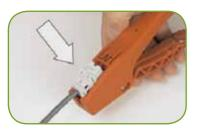
Put the assembly in the universal comfort tool (with the "N" marking) and close it.
