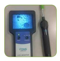
While the expanding beam of the light exiting the fibre makes it less of an issue for direct viewing, using a fibre inspection microscope can be a problem. This hypothesis has been tested, and can confirm that a microscope will focus virtually all the light back into the eye. Many microscopes used in fibre optics, therefore, have filters to absorb any infrared (IR) light that could be harmful. Be wary of inexpensive microscopes, which may not have IR blocking filters.
