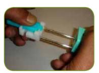
• Check the fibre has not been damaged by the stripping operation by bending the fibre 60 degrees both up and down and left and right. If the fibre breaks start all over again
