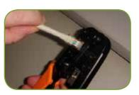
After crimping, inspect the connector to ensure the cable sheath has been correctly inserted into the connector body and the strain relief bar is pressing onto the cable sheath and not to the wires
