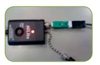
• Connect one cable end to the light source, and then switch it on
