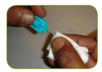
• Clean the stripped fibre with a suitable solvent and a lint free pad. The cleaning should continue until the fibre squeaks while being cleaned. This indicates the fibre is clean and ready for the next step
