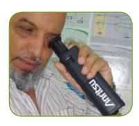
Finally, there is an issue of wavelength. Your eye cannot see many of the wavelengths used in fibre optics because the eye is sensitive to light in the blue to red region of the spectrum while fibre optic systems operate in the infrared. The liquid in your eye which is mostly water absorbs light in the infrared heavily. Light from most fibre optic sources will be absorbed by this liquid, so any potential harm is likely to come to the lens or cornea, not the retina.
