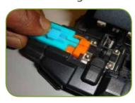
• Mount the cable holder containing the cable clamp assembly into the fibre cleaver. Ensure the end of the fibre coating is in line with the edge of the spacer. Close the cleaver using a smooth action once only
