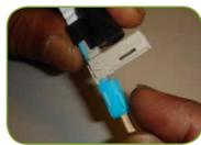
• Ensure there is no gap as shown and that the fibre bend does not extend above the top of the cable clamp
