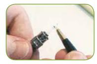
Most cleavers used for splicing or terminating pre-polished/splice connectors hold the fibre after cleaving, so the only problem is disposing of it. It is recommended to use disposable containers like those used for soups at carry-out restaurants. Use it for all your fibre scraps and then seal it and dispose of it properly.
