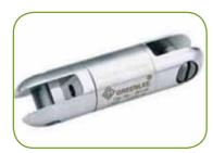
• For pulling the fibre using draw rope, expose and bend the steel strength members to form two hooks, and tape it firmly on the swivel link pulling shackle. This pulling shackle will prevent cable from twisting and damaging the fibre core
