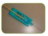
• Mount the cable clamp in the cable holder, ensuring there is no gap between the end of the cable clamp and the corresponding hole in the cable holder
