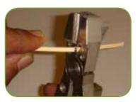
• Strip 50mm of the cable jacket by cutting the tension member and removing the cable sheath with an appropriate tool
