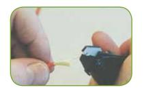
Be extremely careful whenever handling fibres, especially when stripping fibre or scribing and breaking fibre extending out of an adhesive connector. Instead of breaking it, scribe it gently, and then slide your fingers up the connector ferrule, grasping the fibre and pulling it off. Then dispose of it carefully.
