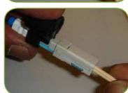
Cable clamp locked in position.
