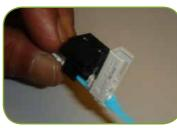
• Holding the connector in both hands verify that the front edge followed by the rear edge of the wedge unit is engaged. This is done by pressing the top and bottom of the wedge unit. If a "Click" is heard then the wedge is Not properly engaged
